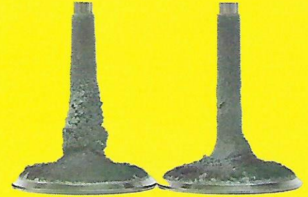
UNTREATED CARBON DEPOSITS
